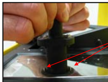
Align new source with 2 pins and tighten 3 screws.
