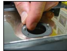
Replace source gasket And screw o-rings.
